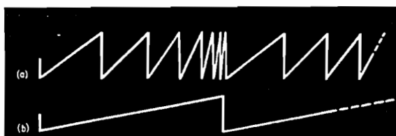
Fig. 4.8(a). Programmed ramp generator output (b) programming waveform
