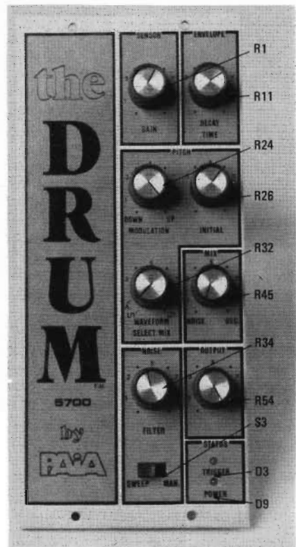
FIG. 9—THE FRONT PANEL of the 5700 synthesizer module with the codes keyed to the various controls.
