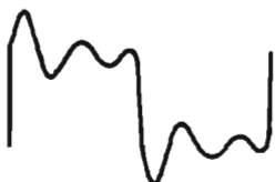
FIG. 15—RINGING WAVEFORM produced by a saxophone excited by a square wave.
