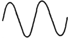
FIG. 14—SINE WAVE contains no harmonics and is a pure tone. It is not produced by natural instruments.
